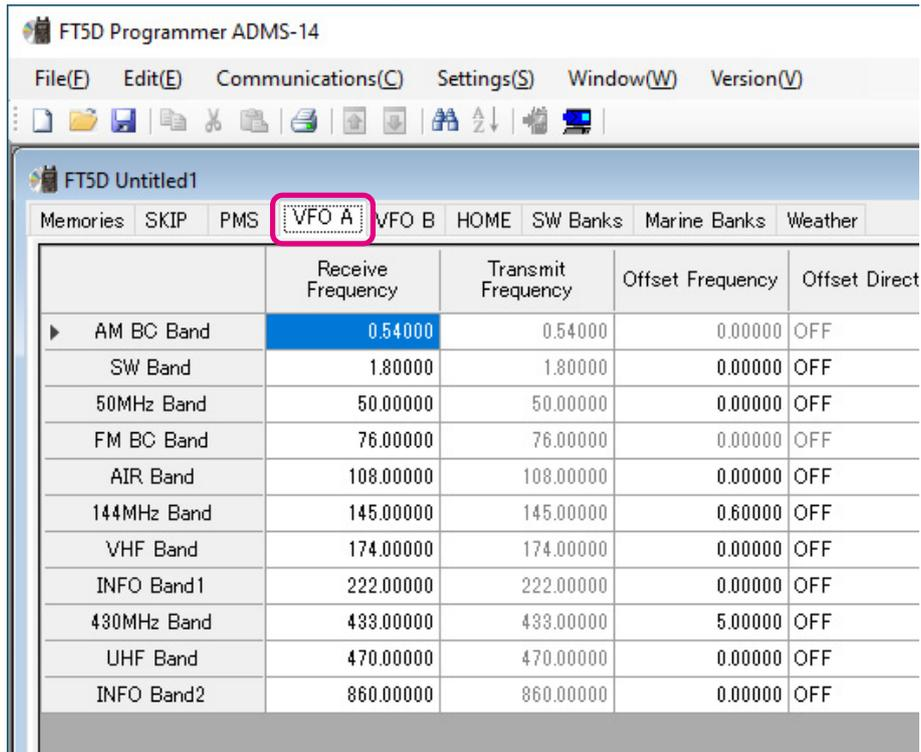
The screenshot shows the FT5D Programmer ADMS-14 software interface. The 'VFO A' tab is selected and highlighted with a red box. The main window displays a table with the following data:
