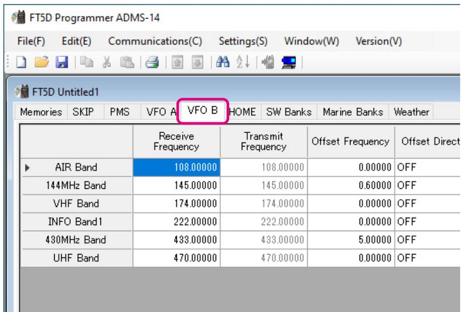
The screenshot shows the FT5D Programmer ADMS-14 software interface. The 'VFO B' tab is selected and highlighted with a red box. The main window displays a table with the following data:
