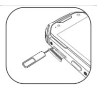
**3** Place the metal side of the Nano card or the Micro SD card face down, at an oblique angle to the bevel of the card, and place it in the card slot as indicated by the arrow in the illustration.
