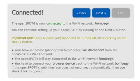
Click on the **Next** button. The openSPOT4 will turn off it's Wi-Fi network "openSPOT4 AP", and its Status LED will become green or alternating green and orange which means the Null connector is active and the device is connected to the selected Wi-Fi network.
