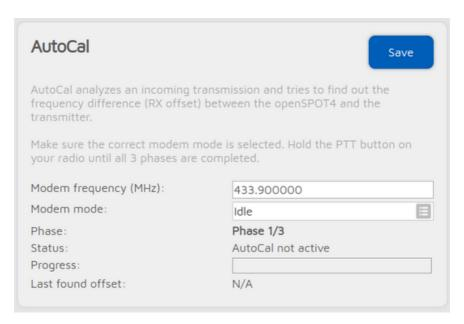
AutoCal is a special connector - it does not connect to anywhere. It analyzes an incoming transmission from the modem and tries to find out the frequency difference (RX offset) between the openSPOT4 and the transmitter.
